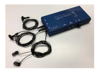
Photo of SignalMaster device showing dual microphones and stereo headphones connected to the system. The system can use any standard 8-12 ohm headphones.
