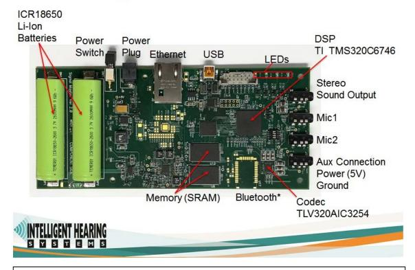
Photo of inside of SignalMaster enclosure showing DSP circuit board, battery charging circuit board, power switch, and power, microphone, headphone connectors.
